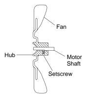
Figure 10 - Fan Cross Section
